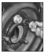
10. Replace the wheel nuts with the rounded end of the nuts toward the wheel. Tighten each nut by hand or with the wheel wrench until the wheel is held against the hub.
